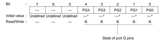
Note: \* Determined by the state of pins PG<sub>4</sub> to PG<sub>0</sub>.
