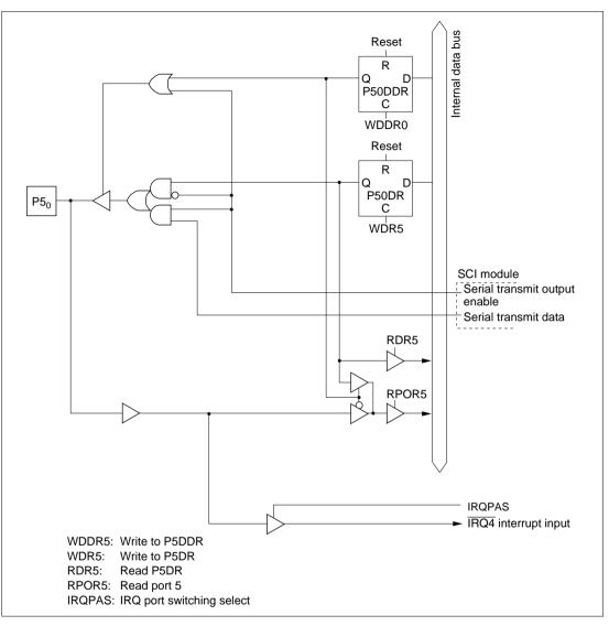
Figure 5.31 (a) Port 5 Block Diagram (Pin P5<sub>0</sub>)
