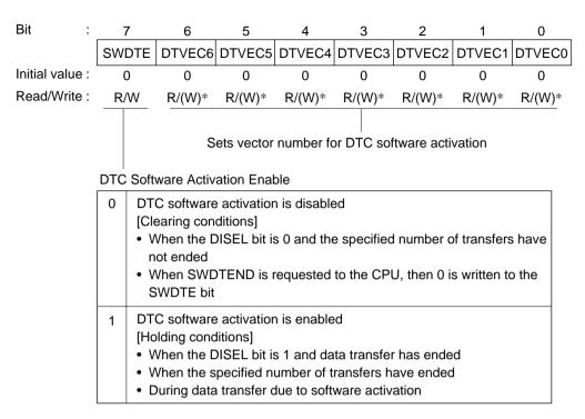
Note: \* DTVEC6 to DTVEC0 bits can be written to when SWDTE = 0.
