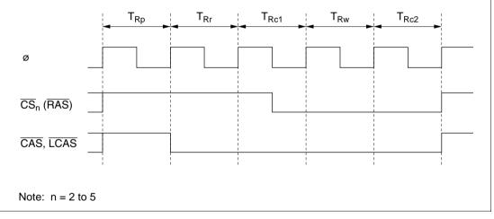
Figure 4.16 CBR Refresh Timing (When RCW = 1, RLW1 = 0, RLW0 = 1)
