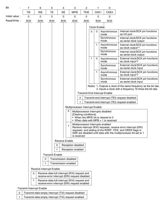
SCR2—Serial Control Register 2
