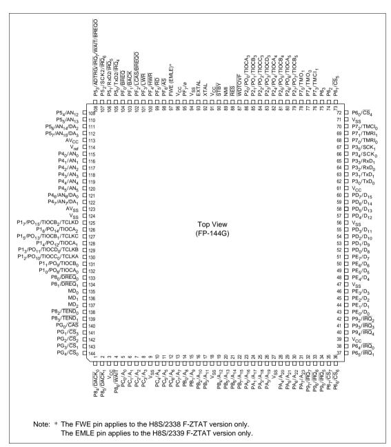
Figure 1.2 shows the pin arrangement of the H8S/2339 and H8S/2338 Series.
