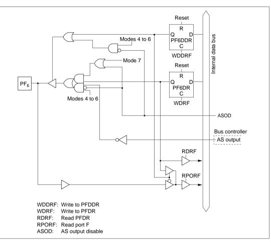
Figure 5.41 (g) Port F Block Diagram (Pin PF<sub>6</sub>)
