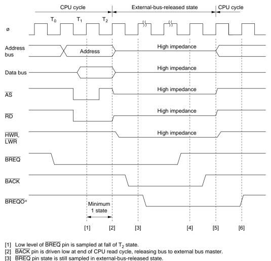
Figure 4.27 shows the timing for transition to the bus-released state.
