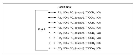
Figure 5.2 Port 2 Pin Functions
