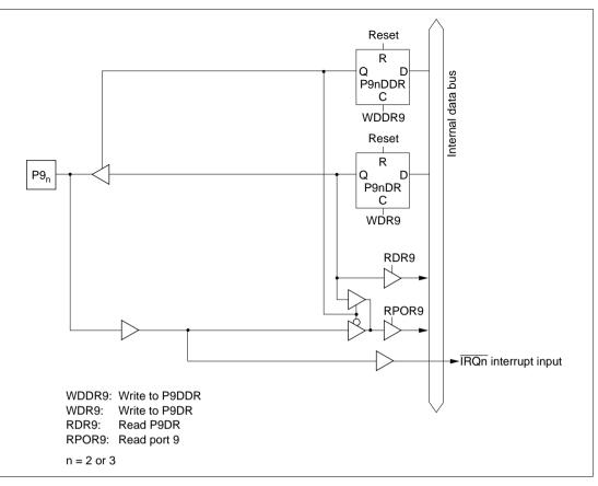
Figure 5.35 (b) Port 9 Block Diagram (Pins P9<sub>2</sub> and P9<sub>3</sub>)
