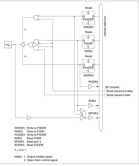
Figure 5.29 (a) Port 3 Block Diagram (Pins P3<sub>0</sub> and P3<sub>1</sub>)
