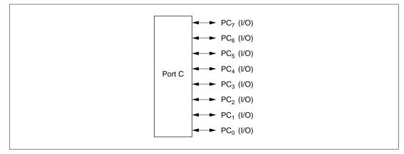
Figure 5.18 Port C Pin Functions (Mode 7)
