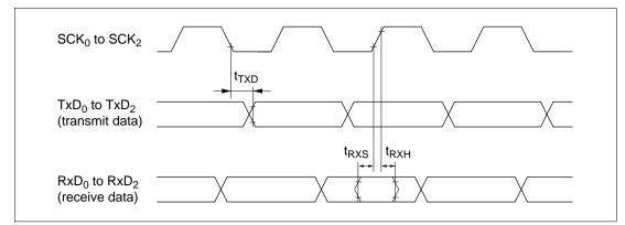
Figure 7.29 SCI Input/Output Timing (Synchronous Mode)
