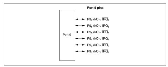
Figure 5.9 Port 9 Pin Functions
