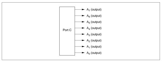
Figure 5.16 Port C Pin Functions (Modes 4 and 5)
