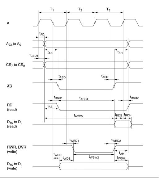
Figure 7.7 Basic Bus Timing (3-State Access)
