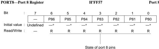
Note: \* Determined by the state of pins P8<sub>6</sub> to P8<sub>0</sub>.
