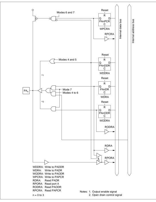
Figure 5.36 (a) Port A Block Diagram (Pins PA<sub>0</sub>, PA<sub>1</sub>, PA<sub>2</sub>, and PA<sub>3</sub>)
