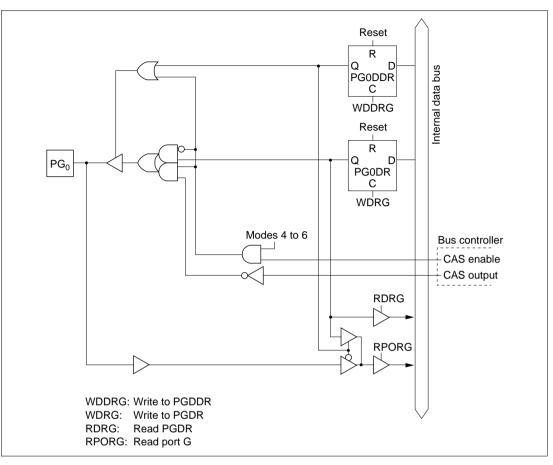
Figure 5.42 (a) Port G Block Diagram (Pin PG<sub>0</sub>)
