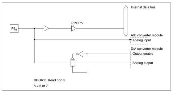
Figure 5.31 (f) Port 5 Block Diagram (Pins  $P5_6$  and  $P_7$ )
