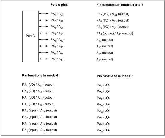
Figure 5.10 Port A Pin Functions
