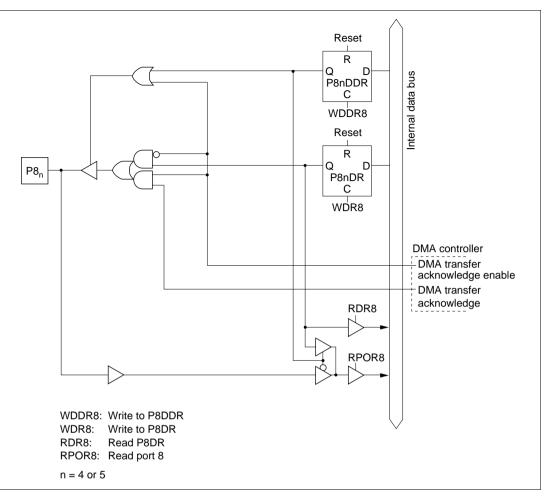
Figure 5.34 (c) Port 8 Block Diagram (Pins P8<sub>4</sub> and P8<sub>5</sub>)
