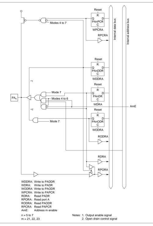
Figure 5.36 (c) Port A Block Diagram (Pins PA<sub>5</sub>, PA<sub>6</sub>, and PA<sub>7</sub>)
