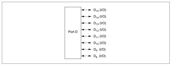
Figure 5.20 Port D Pin Functions (Modes 4 to 6)
