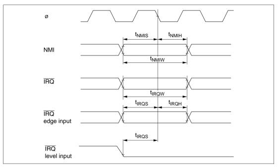
Figure 7.5 Interrupt Input Timing
