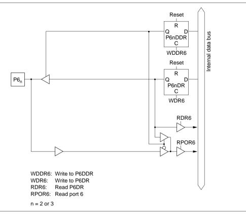
Figure 5.32 (b) Port 6 Block Diagram (Pins P6<sub>2</sub> and P6<sub>3</sub>)
