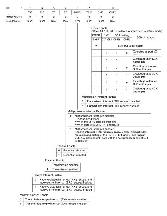
SCR0—Serial Control Register 0
