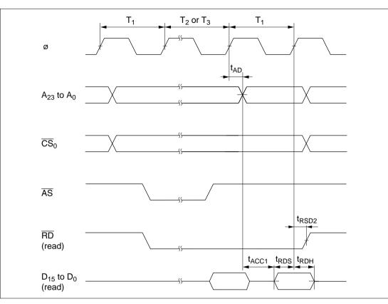
Figure 7.13 Burst ROM Access Timing (1-State Access)
