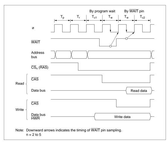
Figure 4.7 shows an example of wait state insertion timing.
