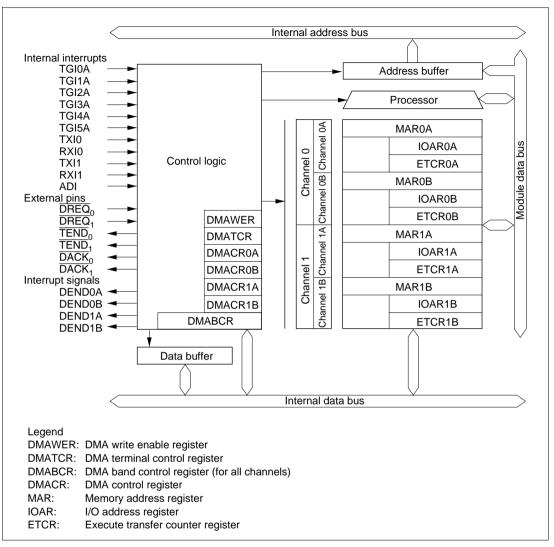
Figure 6.2 Block Diagram of DMAC
