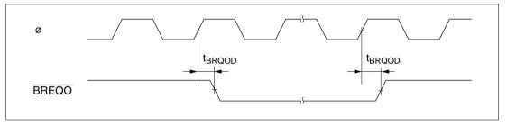
Figure 7.15 External Bus Request Output Timing
