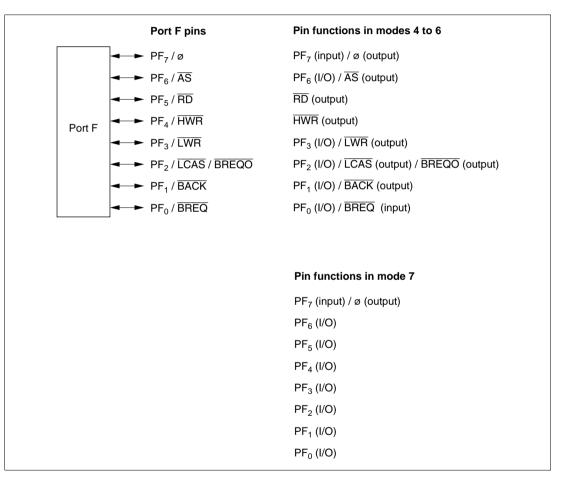
Figure 5.25 Port F Pin Functions
