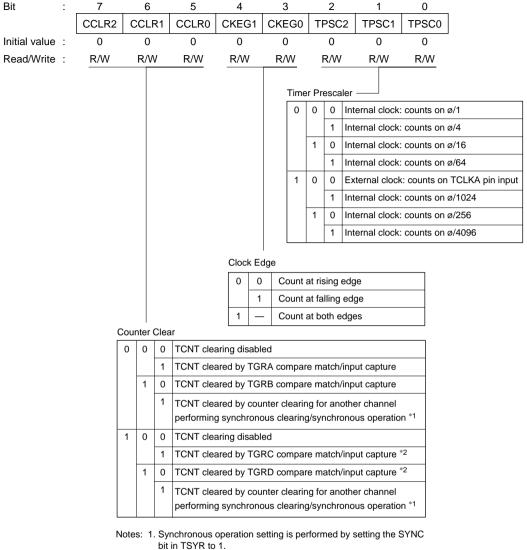
When TGRC or TGRD is used as a buffer register, TCNT is not cleared because the buffer register setting has priority, and compare match/input capture does not occur.
