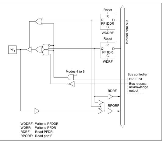
Figure 5.41 (b) Port F Block Diagram (Pin PF<sub>1</sub>)
