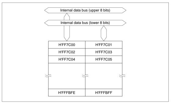
Figure 6.12 Block Diagram of RAM (32 kbytes)
