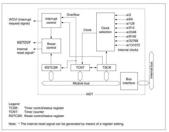
Figure 6.7 Block Diagram of WDT
