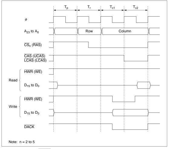
Figure 4.18 DACK Output Timing when DDS = 1 (Example of DRAM Access)
