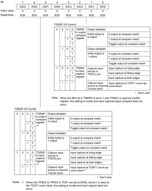
When the BFB bit in TMDR0 is set to 1 and TGR0D is used as a buffer register, this setting is invalid and input capture/output compare does not occur.
