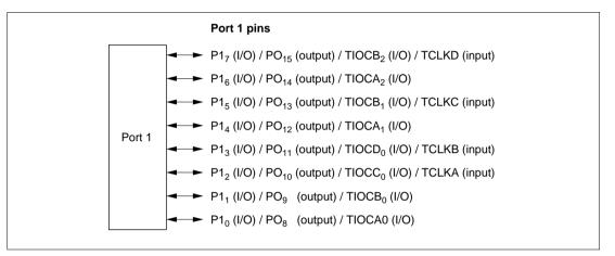
Figure 5.1 Port 1 Pin Functions
