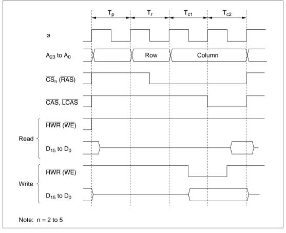
Figure 4.5 Basic Access Timing
