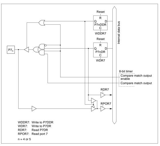
Figure 5.33 (c) Port 7 Block Diagram (Pins P7<sub>4</sub> and P7<sub>5</sub>)
