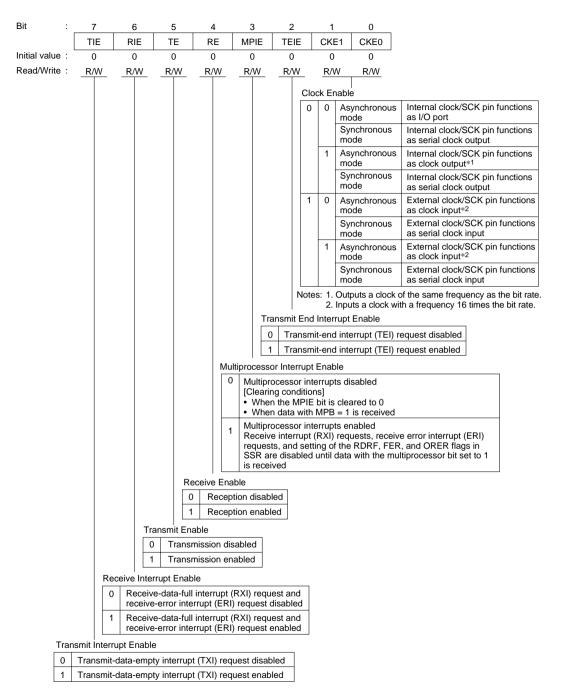
SCR1—Serial Control Register 1
