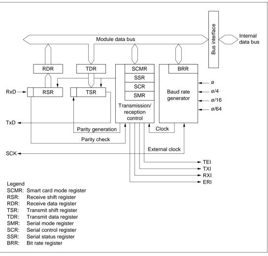
Figure 6.8 Block Diagram of SCI
