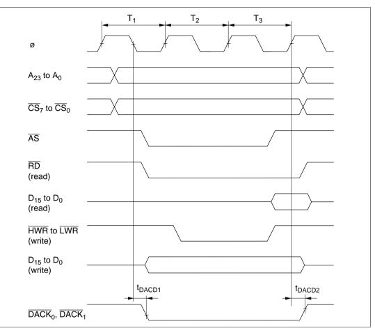
Figure 7.17 DMAC Single Address Transfer Timing (3-State Access)
