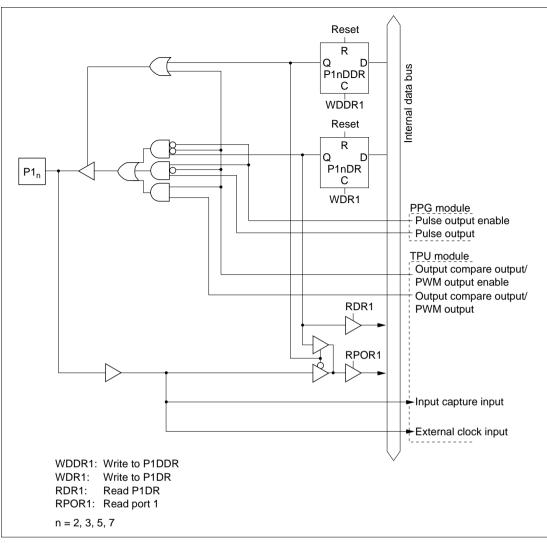
Figure 5.27 (b) Port 1 Block Diagram (Pins P1<sub>2</sub>, P1<sub>3</sub>, P1<sub>5</sub>, and P1<sub>7</sub>)
