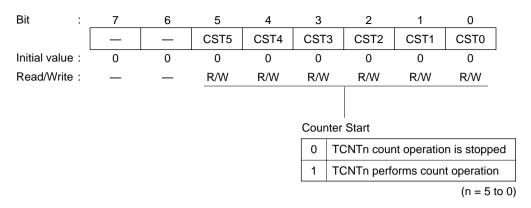
Note: If 0 is written to the CST bit during operation with the TIOC pin designated for output, the counter stops but the TIOC pin output compare output level is retained. If TIOR is written to when the CST bit is cleared to 0, the pin output level will be changed to the set initial output value.
