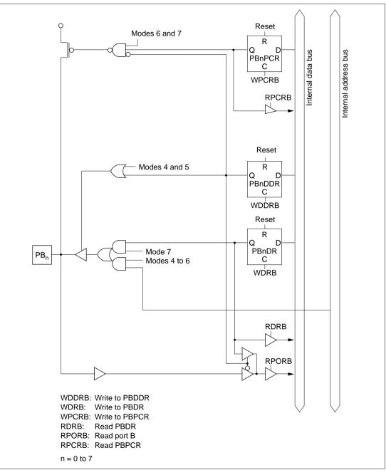
Figure 5.37 Port B Block Diagram (Pins PB<sub>n</sub>)
