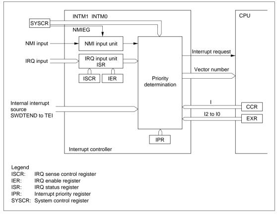
Figure 6.1 Block Diagram of Interrupt Controller
