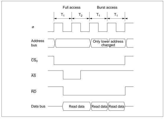
Figure 4.20 (b) Example of Burst ROM Access Timing (When AST0 = BRSTS1 = 0)
