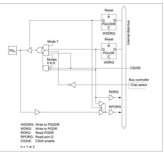
Figure 5.42 (b) Port G Block Diagram (Pins PG<sub>1</sub> and PG<sub>2</sub>)
