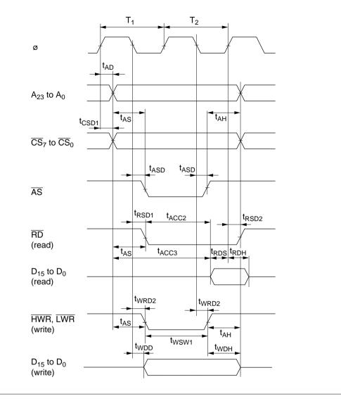
Figure 7.6 Basic Bus Timing (2-State Access)
