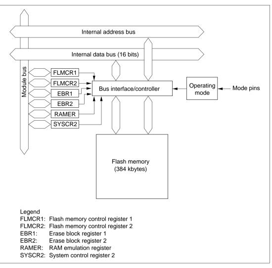
Figure 6.15 Block Diagram of Flash Memory
