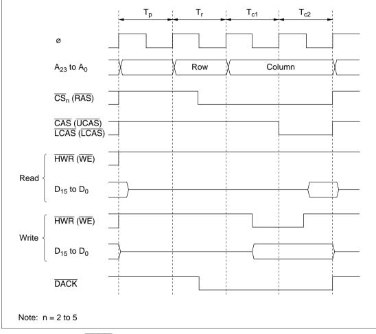
Figure 4.19 DACK Output Timing when DDS = 0 (Example of DRAM Access)
