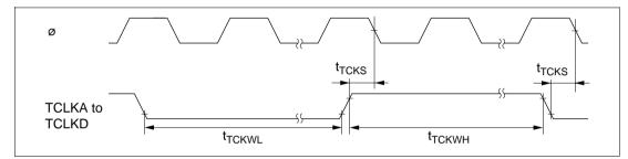
Figure 7.23 TPU Clock Input Timing
