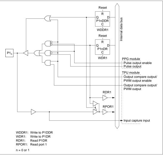
Figure 5.27 (a) Port 1 Block Diagram (Pins P1<sub>0</sub> and P1<sub>1</sub>)
