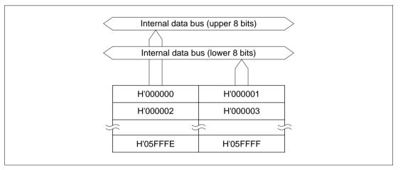
Figure 6.14 Block Diagram of Flash Memory (384 kbytes)
