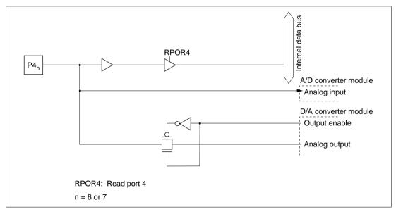
Figure 5.30 (b) Port 4 Block Diagram (Pins P4<sub>6</sub> and P4<sub>7</sub>)
