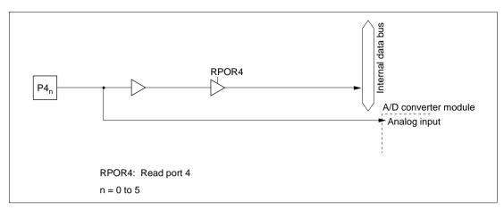
Figure 5.30 (a) Port 4 Block Diagram (Pins P4<sub>0</sub> to P4<sub>5</sub>)
