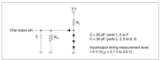
Figure 7.1 Output Load Circuit
