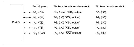
Figure 5.26 Port G Pin Functions
