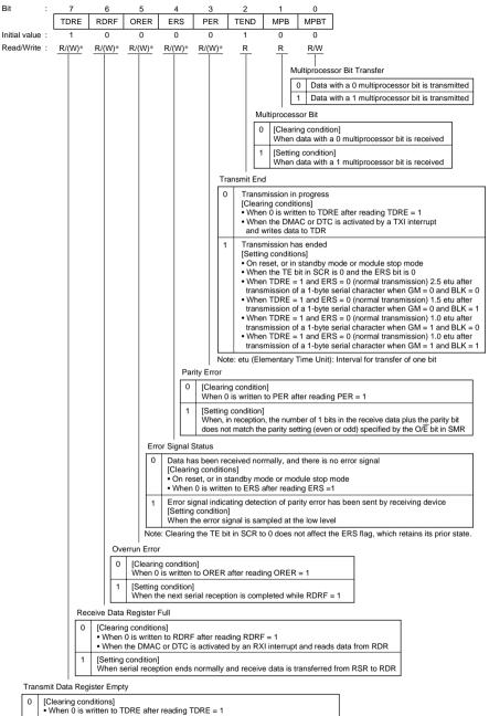
When the DMAC or DTC is activated by a TXI interrupt and writes data to TDR
