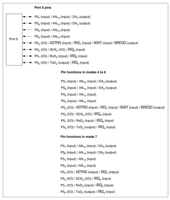
Figure 5.5 Port 5 Pin Functions
