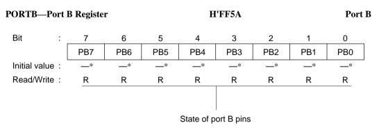
Note: \* Determined by the state of pins  $PB_7$  to  $PB_0$ .
