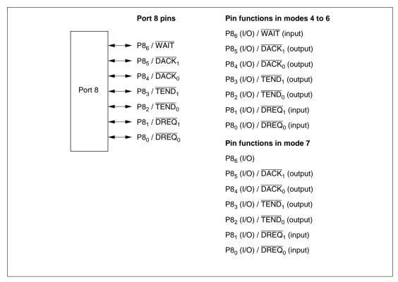
Figure 5.8 Port 8 Pin Functions
