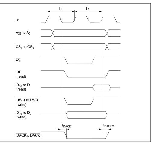
Figure 7.16 DMAC Single Address Transfer Timing (2-State Access)
