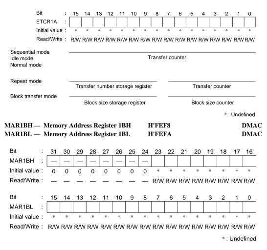
In short address mode: Specifies transfer source/transfer destination address In full address mode: Transfer destination address
