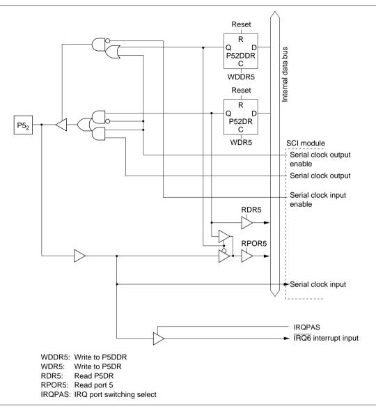
Figure 5.31 (c) Port 5 Block Diagram (Pin P5<sub>2</sub>)
