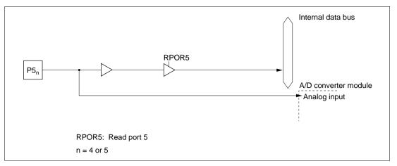
Figure 5.31 (e) Port 5 Block Diagram (Pins P5<sub>4</sub> and P<sub>5</sub>)
