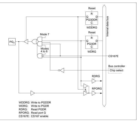
Figure 5.42 (c) Port G Block Diagram (Pin PG<sub>3</sub>)
