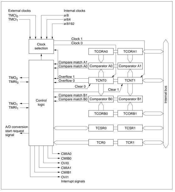
Figure 6.6 Block Diagram of 8-Bit Timer
