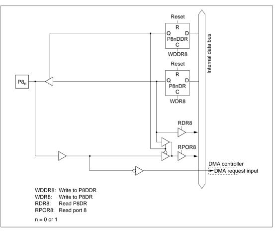
Figure 5.34 (a) Port 8 Block Diagram (Pins P8<sub>0</sub> and P8<sub>1</sub>)
