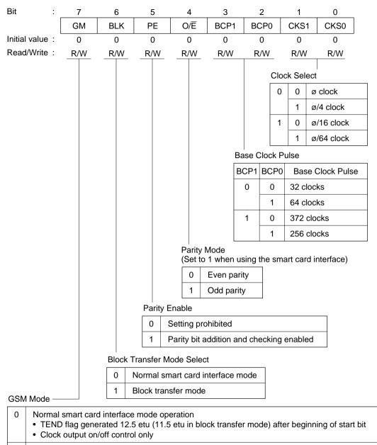
GSM mode smart card interface mode operation
