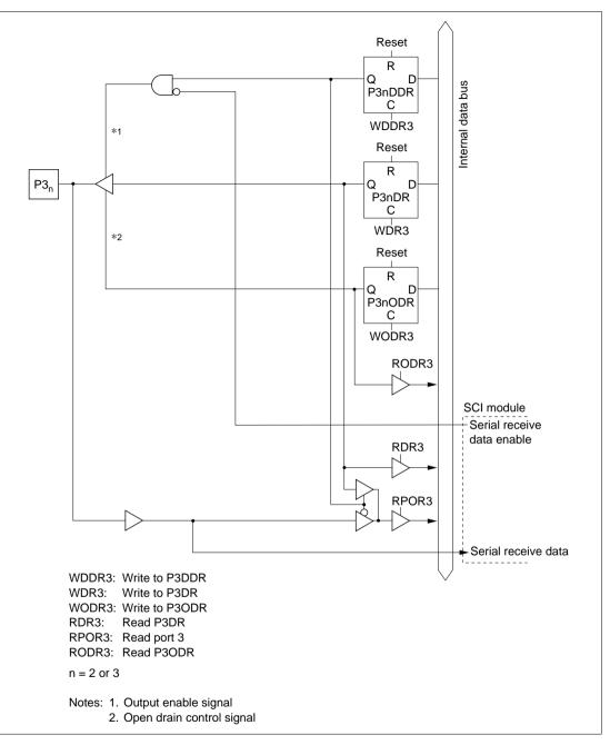
Figure 5.29 (b) Port 3 Block Diagram (Pins P3<sub>2</sub> and P3<sub>3</sub>)
