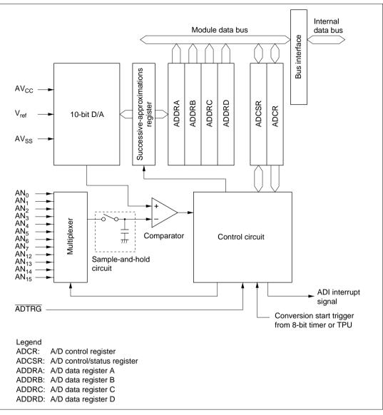
Figure 6.10 Block Diagram of A/D Converter
