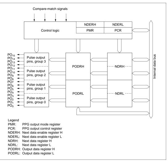
Figure 6.5 Block Diagram of PPG
