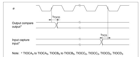
Figure 7.22 TPU Input/Output Timing
