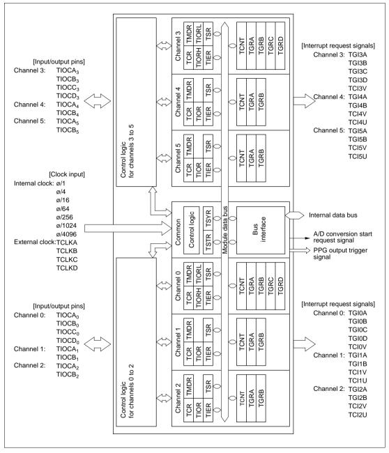
Figure 6.4 Block Diagram of TPU
