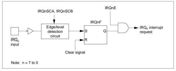
Figure 3.1 Block Diagram of Interrupts IRQ<sub>7</sub> to IRQ<sub>0</sub>
