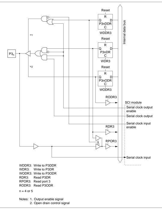
Figure 5.29 (c) Port 3 Block Diagram (Pins P3<sub>4</sub> and P3<sub>5</sub>)
