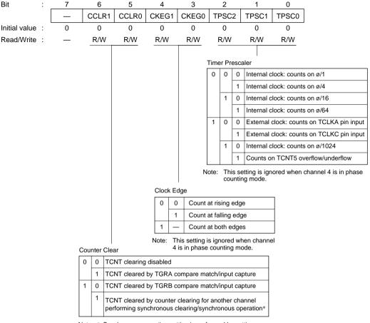
Note: \* Synchronous operation setting is performed by setting the SYNC bit in TSYR to 1.
