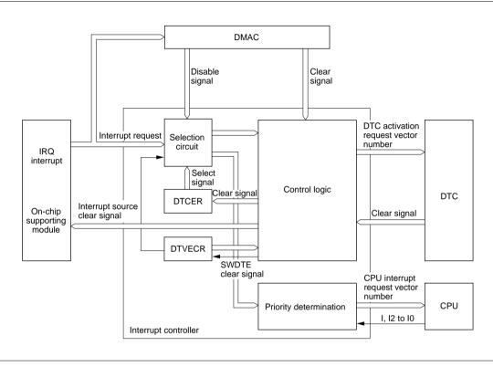
Figure 3.3 shows a block diagram of the DTC, DMAC, and interrupt controller.
