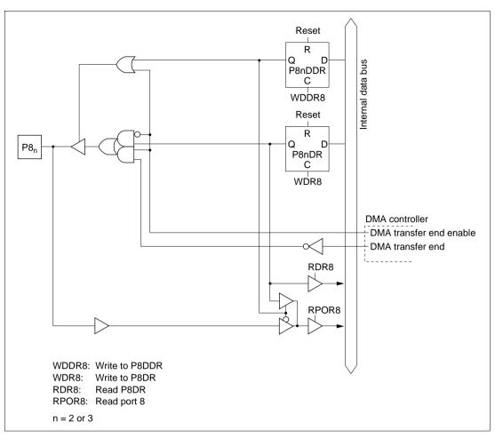
Figure 5.34 (b) Port 8 Block Diagram (Pins P8<sub>2</sub> and P8<sub>3</sub>)
