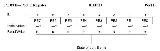
Note: \* Determined by the state of pins PE<sub>7</sub> to PE<sub>0</sub>.
