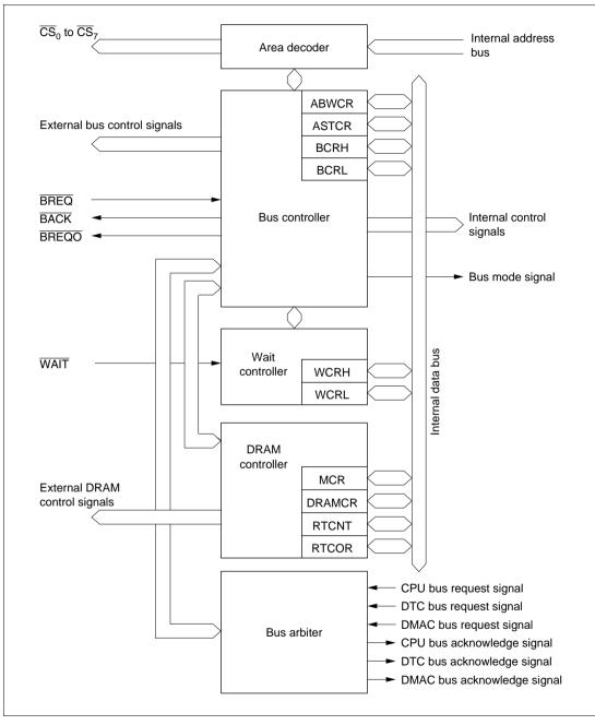
Figure 4.1 Block Diagram of Bus Controller
