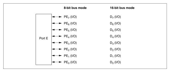
Figure 5.23 Port E Pin Functions (Modes 4 to 6)
