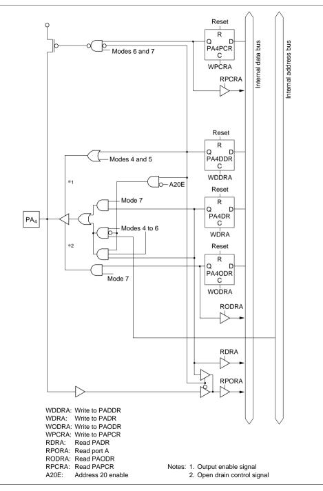
Figure 5.36 (b) Port A Block Diagram (Pin PA<sub>4</sub>)
