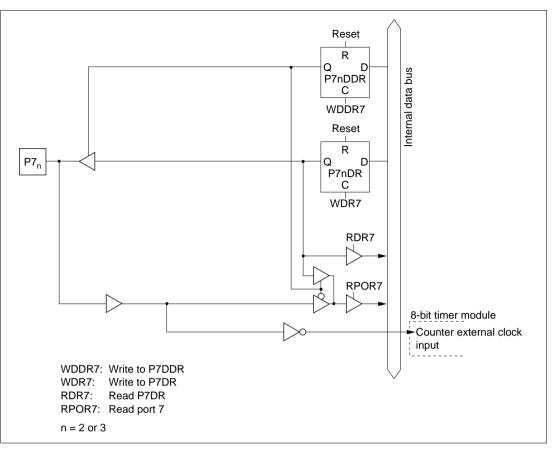
Figure 5.33 (b) Port 7 Block Diagram (Pins P7<sub>2</sub> and P7<sub>3</sub>)
