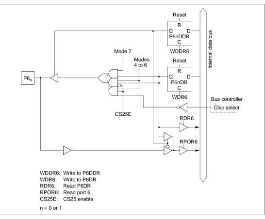
Figure 5.32 (a) Port 6 Block Diagram (Pins P6<sub>0</sub> and P6<sub>1</sub>)
