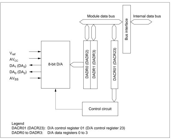
Figure 6.11 Block Diagram of D/A Converter
