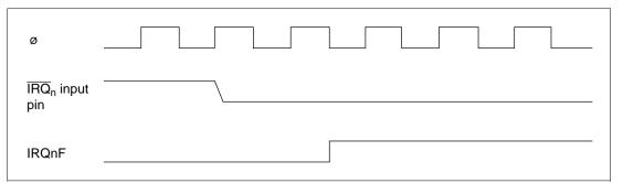
Figure 3.2 Timing of IRQnF Setting
