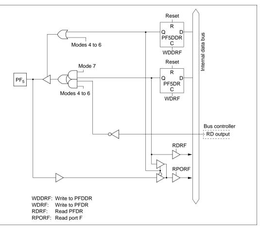
Figure 5.41 (f) Port F Block Diagram (Pin PF<sub>5</sub>)
