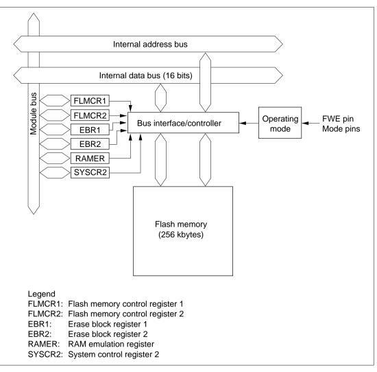
Figure 6.17 Block Diagram of Flash Memory
