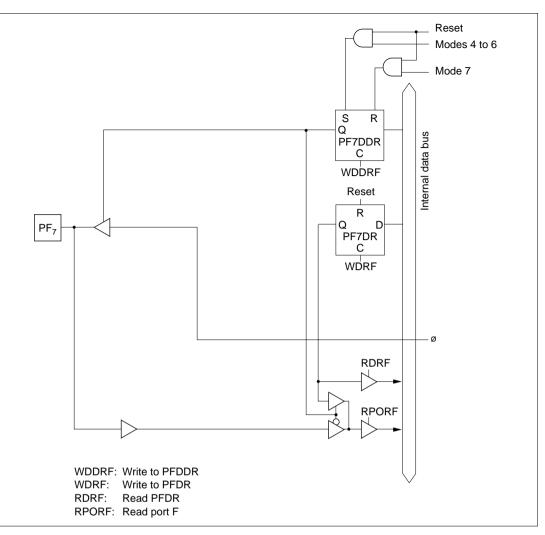
Figure 5.41 (h) Port F Block Diagram (Pin PF<sub>7</sub>)
