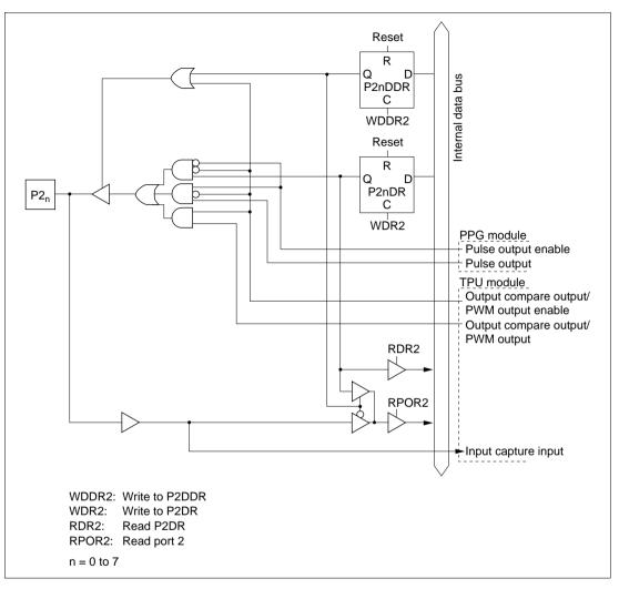
Figure 5.28 Port 2 Block Diagram (Pins P2<sub>n</sub>)
