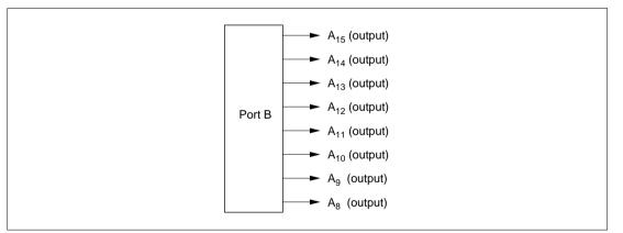
Figure 5.12 Port B Pin Functions (Modes 4 and 5)
