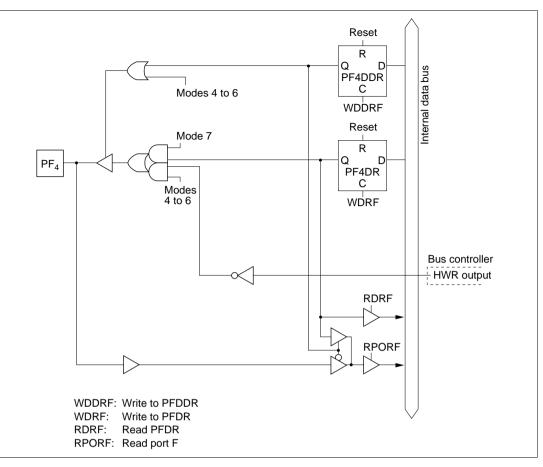
Figure 5.41 (e) Port F Block Diagram (Pin PF<sub>4</sub>)
