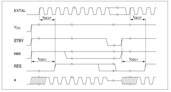
Figure 7.3 Oscillation Stabilization Timing
