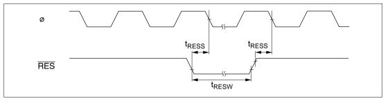
Figure 7.4 Reset Input Timing
