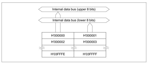
Figure 6.16 Block Diagram of Flash Memory (256 kbytes)
