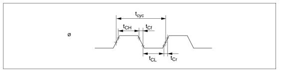
Figure 7.2 System Clock Timing
