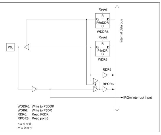
Figure 5.32 (c) Port 6 Block Diagram (Pins P6<sub>4</sub> and P6<sub>5</sub>)
