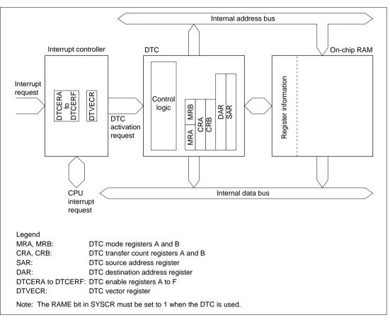
Figure 6.3 Block Diagram of DTC
