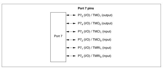
Figure 5.7 Port 7 Pin Functions
