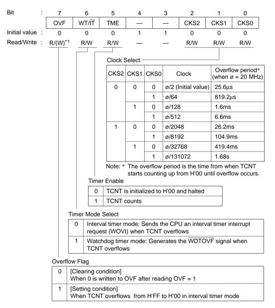
The method for writing to TCSR is different from that for general registers to prevent accidental overwriting. For details, see section 10.2.4, Notes on Register Access, in the Hardware Manual.
