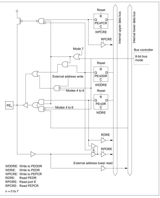
Figure 5.40 Port E Block Diagram (Pins PE<sub>n</sub>)
